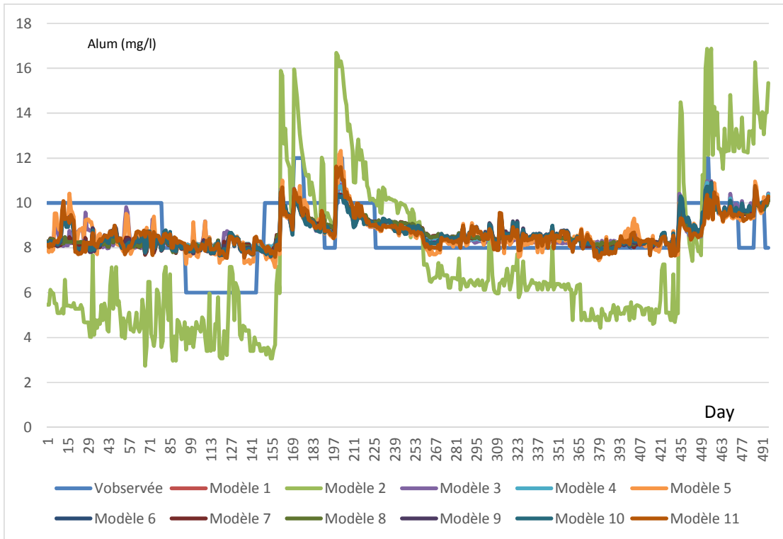
Fig. 6. Simulation of aluminum sulfate dose (mg/l) by different models and dose measured for turbidity less than 10 NTU
