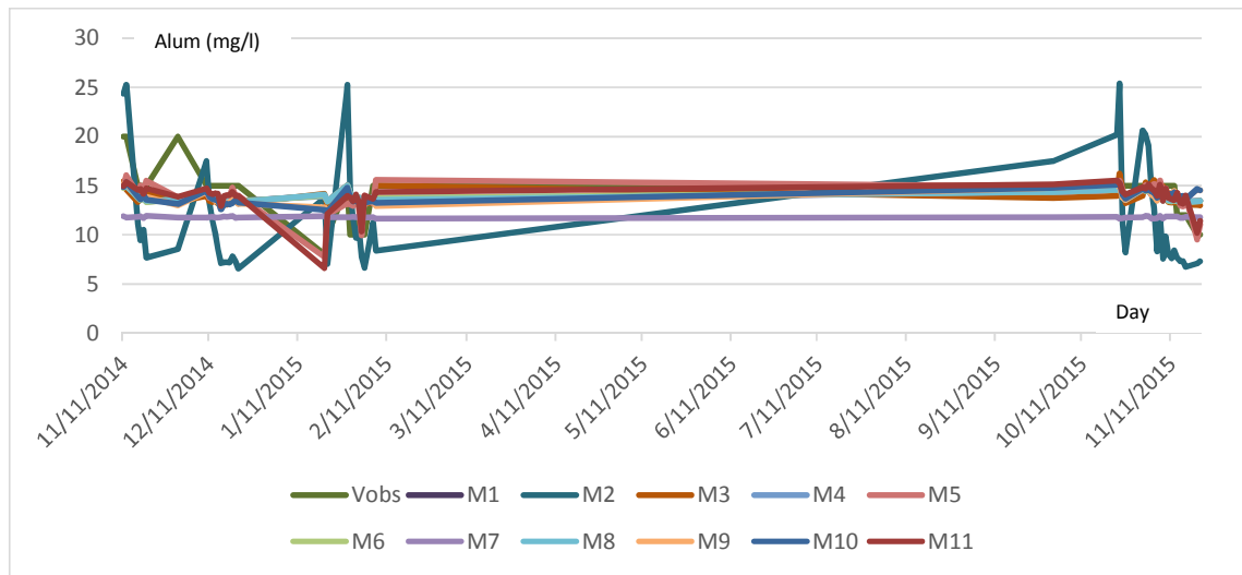
Fig. 8. Simulation of aluminum sulfate dose (mg/l) by different models and dose measured for turbidity between 10 and 20 NTU
