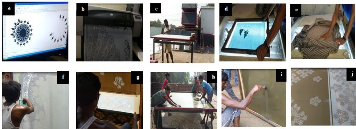
Fig. 4. Steps in screen making
