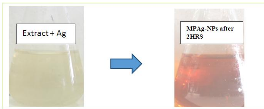
Fig. 1. Color changes observed 2 hours after adding AgNO 3 in the aqueous extract of Mangifera indica
