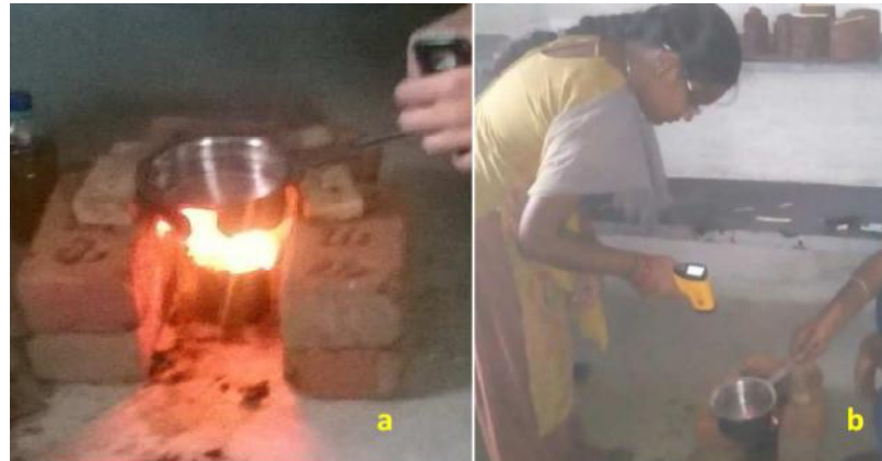
Fig. 8. boiling of water by burning developed briquettes a. Burning of briquettes b. measuring temperature using infra-red thermometer
