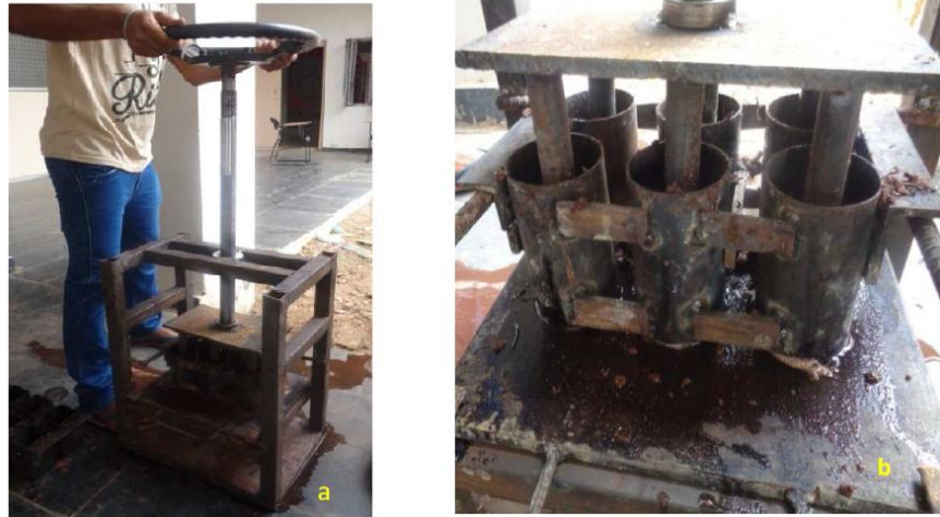
Fig. 6. Production of briquettes with developed machine along with square mould a. Pressing of briquettes, b. A view of pistons inside the respective circular mould
