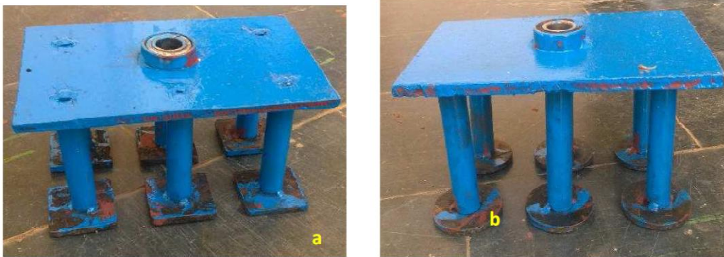
Fig. 3a. Developed square mould pressing plates, b. Developed circular mould pressing plate
