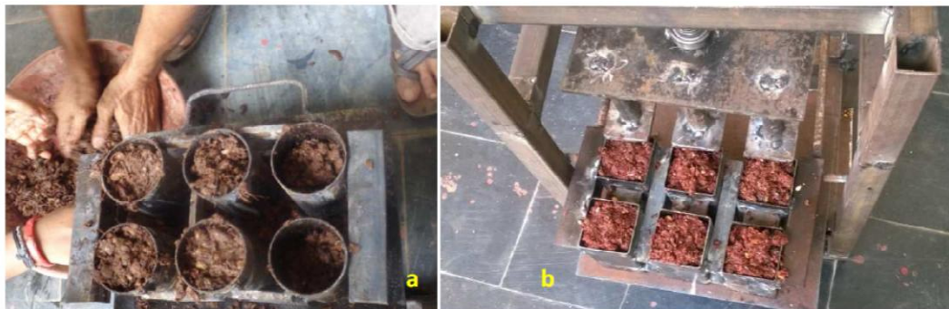
Fig. 5. Loading of slurry in to the developed moulds a. Slurry in circular mould, b. slurry in square mould
