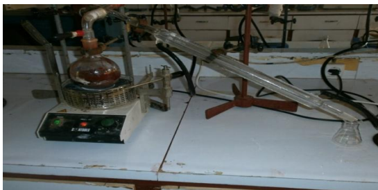
Fig. 2. Pyrolysis experimental set up
