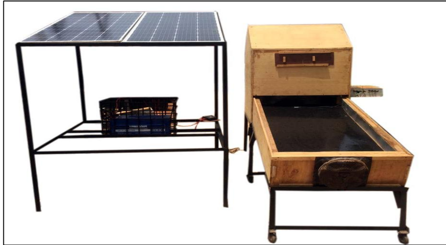
Fig. 3. The developed solar controlled hot-air supplemented dryer
